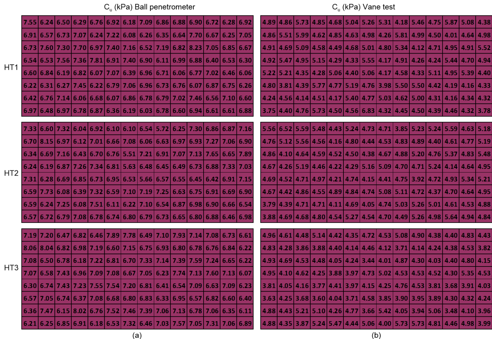
Figure 5.44 Undrained shear strength direct measurements in kPa of homogenous traditional technique models: (a) mini ball penetrometer and (b) mini vane.
