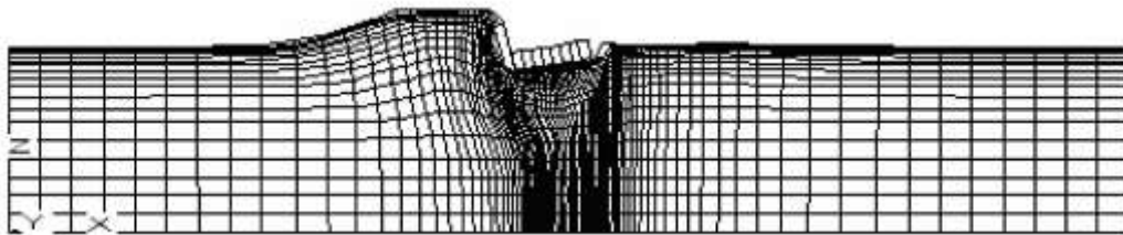
Figure 3.4 Deformed mesh corresponding to a realization of the random soil (Taken from Soubra et al. (2008)).
