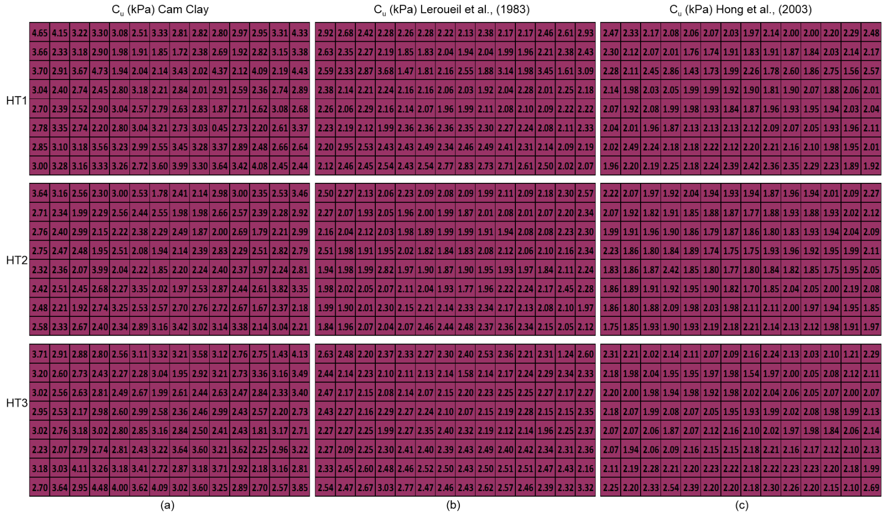
Figure 5.37 Undrained shear strength indirect measurements in kPa for homogeneous models traditional technique: (a) Cam clay theory, (b) Leroueil et al., (1983) and (c) Hong et al., (2003).
