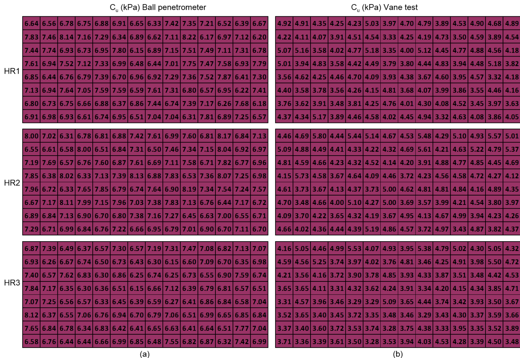
Figure 5.45 Undrained shear strength direct measurements in kPa of homogenous random technique models: (a) mini ball penetrometer and (b) mini vane.
