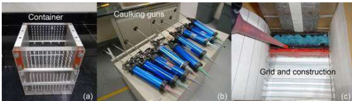
Figure 5.35 Construction of the heterogeneous model: (a) container box with vertical extensions, (b) caulking guns, (c) process of placing the strings of slurries into the container.
