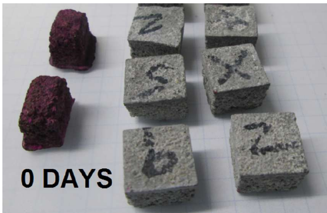
Figure 3.8: Non-carbonated (left) and carbonated samples (right) before exposure. In this picture, non-carbonated have the half of the size of carbonated samples
