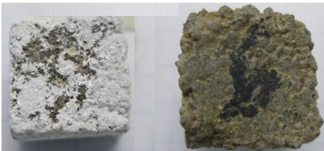
Figure 4.7: Antimicrobial effect of Triclosan in samples inoculated in aseptic conditions after 150 days of exposure. Left: With no additions; Right: Added with Triclosan
