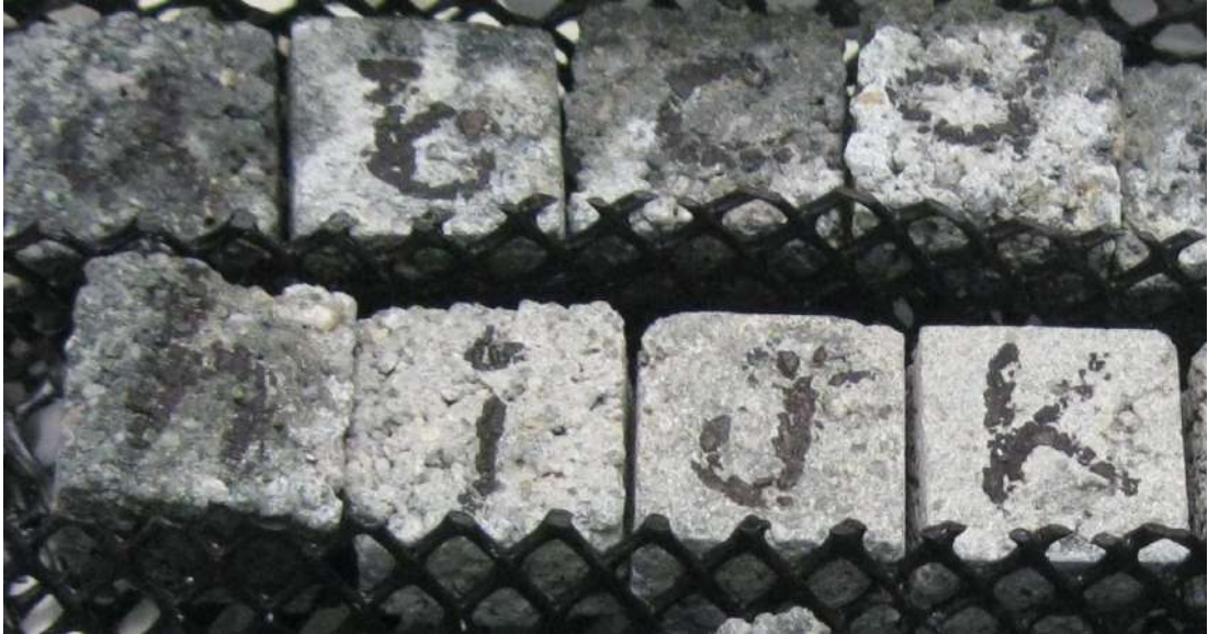
Figure 4.2: Stage of H_2S -only control samples after 153 days of exposure manipulated in non aseptic conditions
