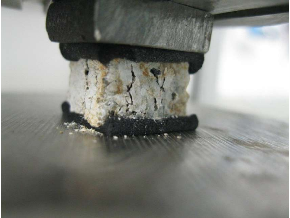
Figure 5.34: Typical compressive breaking of exposed samples
