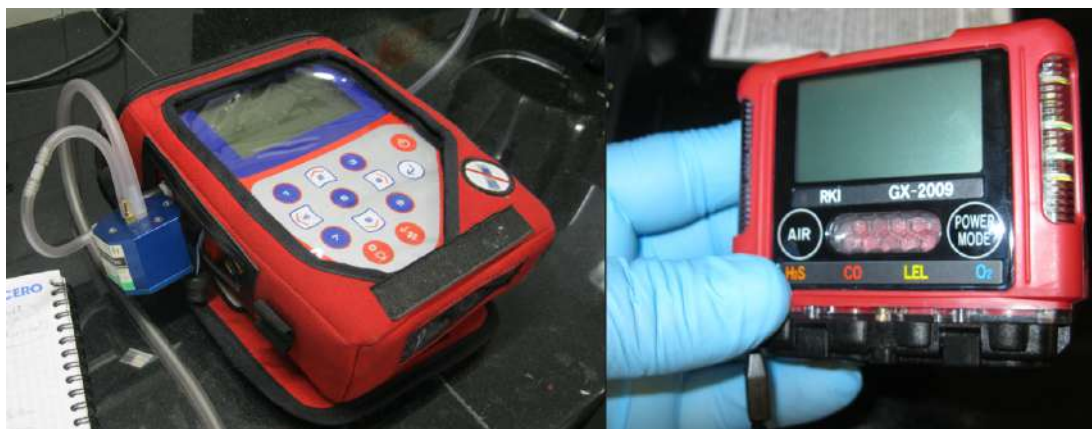
Figure 3.10: Portable Gas Analyzer BioGas CDM (LANDTEC ® ) and RKI GX2009 (RKI Instruments ® )
