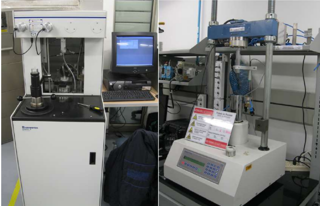
Figure 3.16: AutoPore IV 9500 porosimeter (Micromertics Instrument Corporation ® ) and hydraulic press (ELE International Digital Tritest ® )
