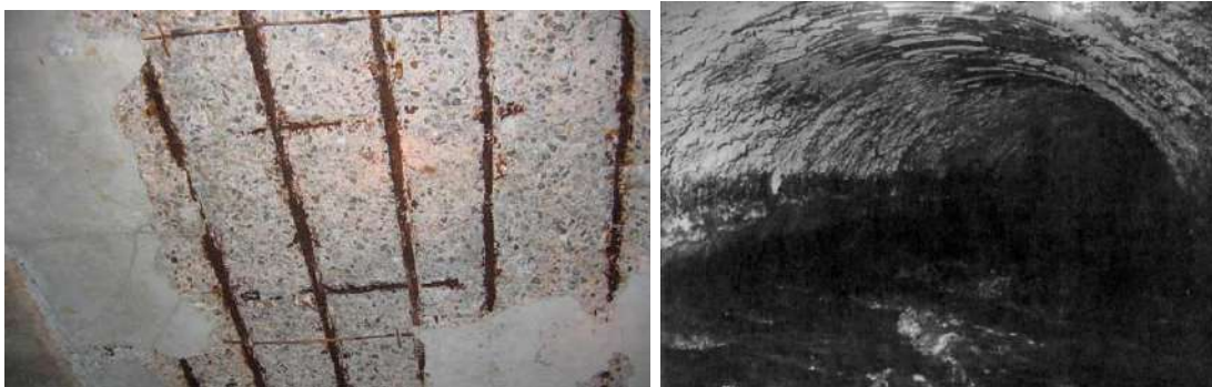
Figure 1.1: Examples of concrete biodeterioration (from http://www.engr.psu.edu ) a) Exposed corroded reinforcement bars. b) Deteriorated concrete in sewer
