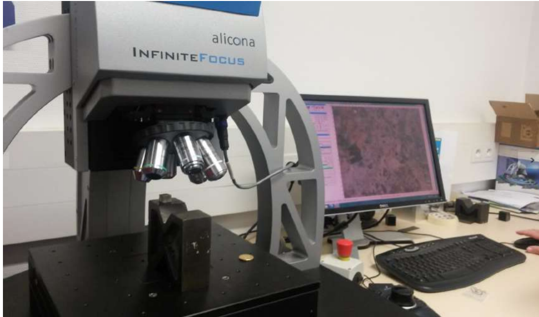
Figure 3.15: Alicona Infinite Focus optical device ®
