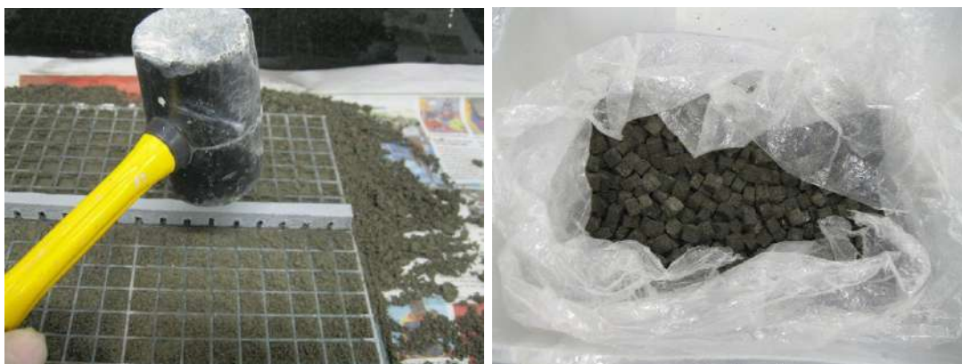
Figure 3.6: Casting and curing of samples
